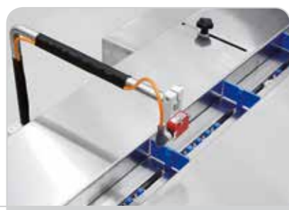
"No Product-No Bag" function detection photocell at in-feed conveyor
