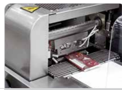
Cross sealing system by rotary sealing head
